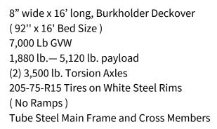
Treated Lumber Floor Stake Pockets and Rub Rail Toolbox in the Tongue Sealed LED Lighting Safety Chains 7,000 lbs. Drop Leg Jack 2-5/16" Ball Coupler 3 Year MFG Warranty
